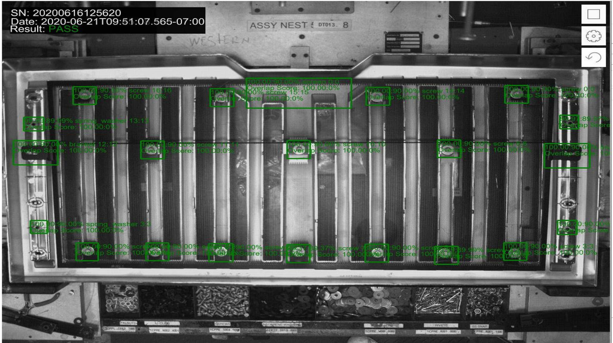
Over 20 components verified for presence on a 6ft wide grill using one camera – note the chrome finish.
