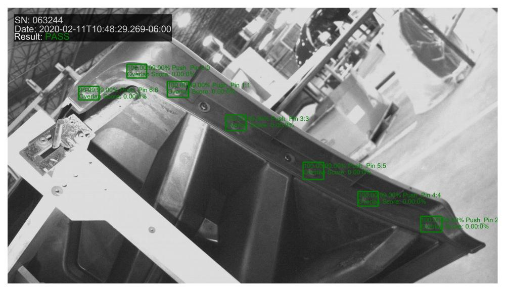
Left side of bumper – part is approximately 40" long with 7 .3125" diameter push pins black on black and two similar looking screws
