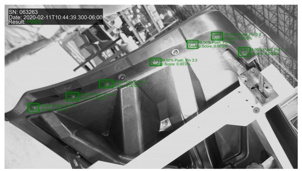
Right side of bumper – part is approximately 40" long with 7 push pins and two similar looking screws. Notice the background of this one is white.
